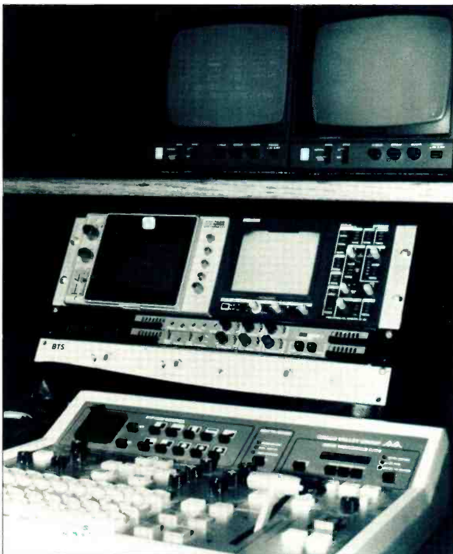
Closeup of Frame Runner's ER1. ER2 is similarly equipped, but uses a Magni WFM560 waveform monitor and VS560 vectorscope.
