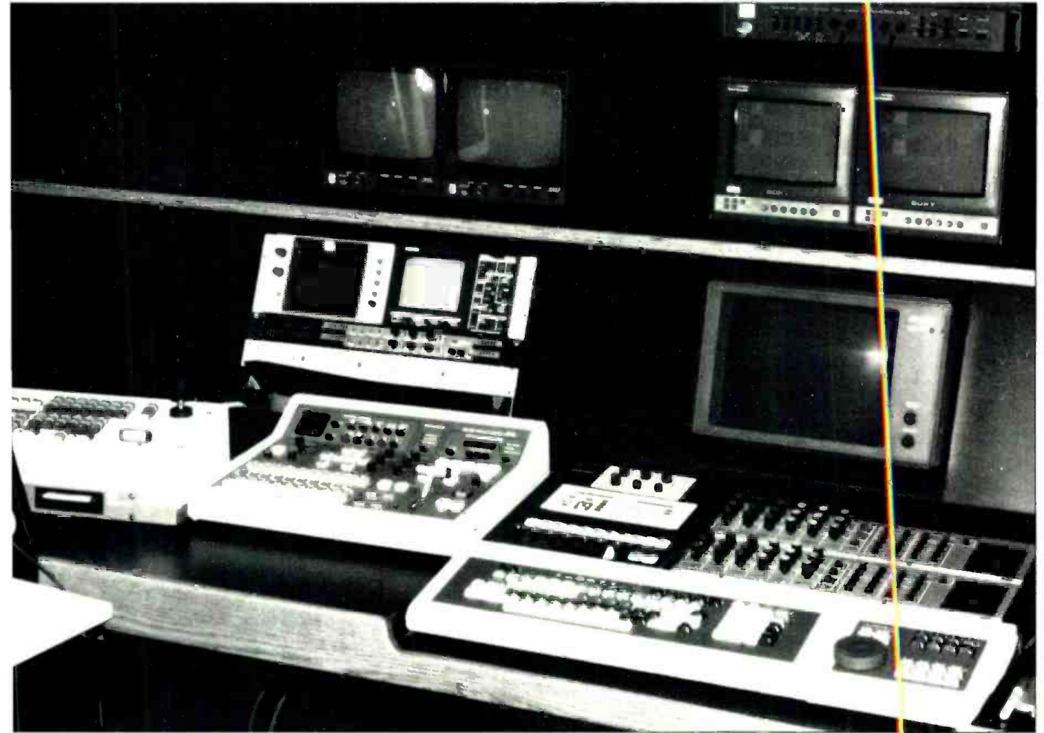
Basic test equipment—a Magni WFM560 waveform monitor and Tektronix 1420 NTSC vectorscope—is integrated into Edit Room 1 at Frame Runner in New York City.
